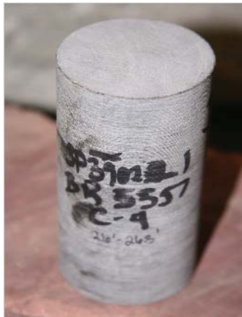
Fig 4: Rock core from 26 ft. to 26.8 ft.
